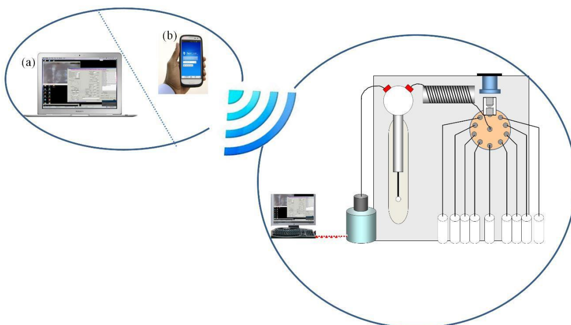
Figure 2. Remote control of the SI- LAV system via the internet with IT devices (a) a laptop computer and (b) a mobile phone.
