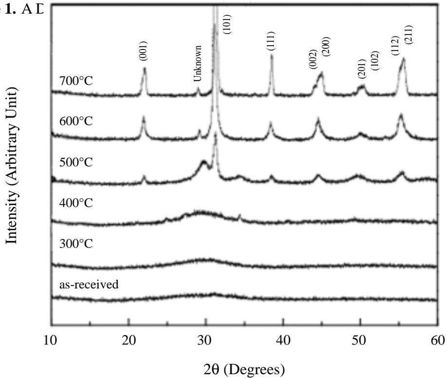
**Figure 2.** X-ray diffraction patterns of as-received PZT powder and PZT powders calcined at 300, 400, 500, 600 and 700°C.
