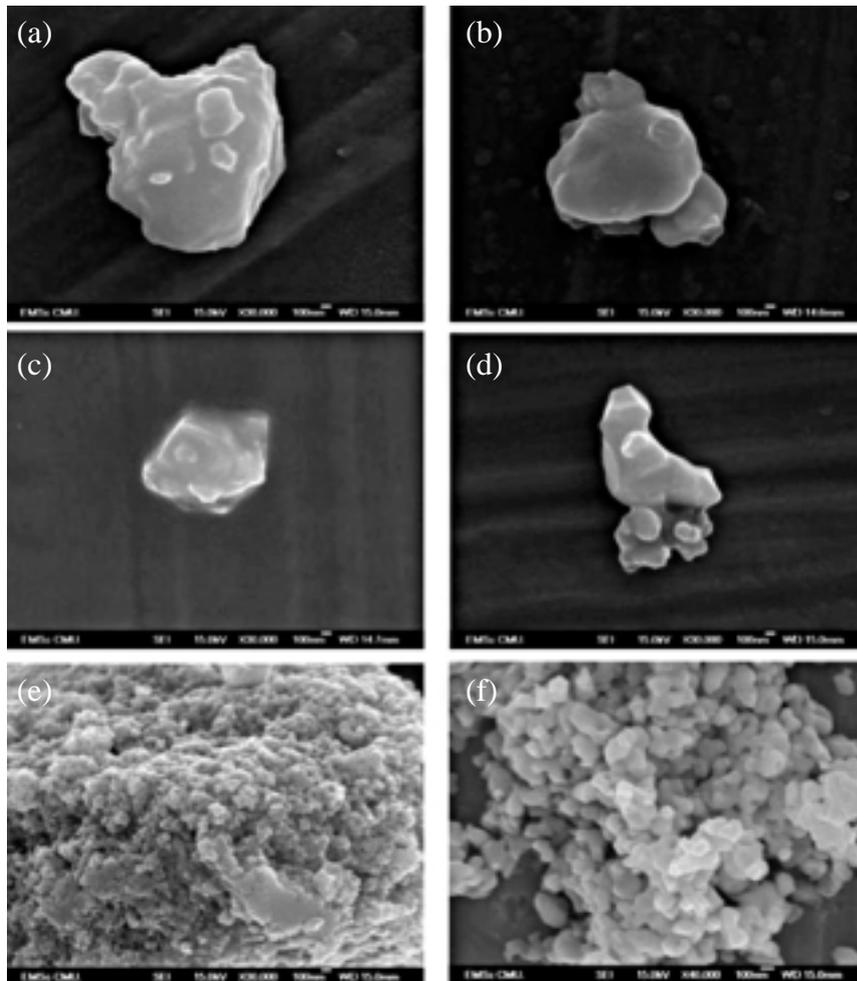
**Figure 3.** SEM micrographs of (a) as-received PZT powder and PZT powders calcined at (b) 300, (c) 400, (d) 500, (e) 600 and (f) 700°C.
