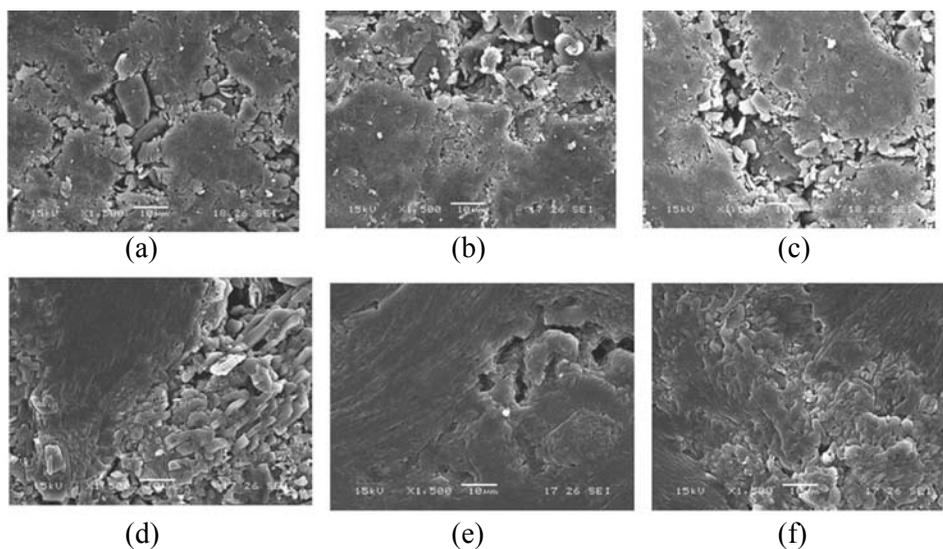
**Figure 3.** The surface morphologies by SEM (1,500X) of the WG blank tablets at CF of (a) 1000 kg, (b) 1400 kg and (c) 1800 kg and of DSDT prepared from WG blank tablet at (d) 1000 kg, (e) 1400 kg and (f) 1800 kg of CF.
