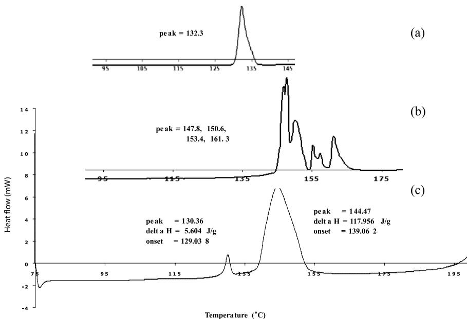
**Figure 9.** DSC thermograms of (a) diazepam, (b) lactose and (c) powder scratched from the surface of DSDT prepared from WG blank tablet of 1000 kg CF. The curves have been separated in the y-axis to aid comparison.
