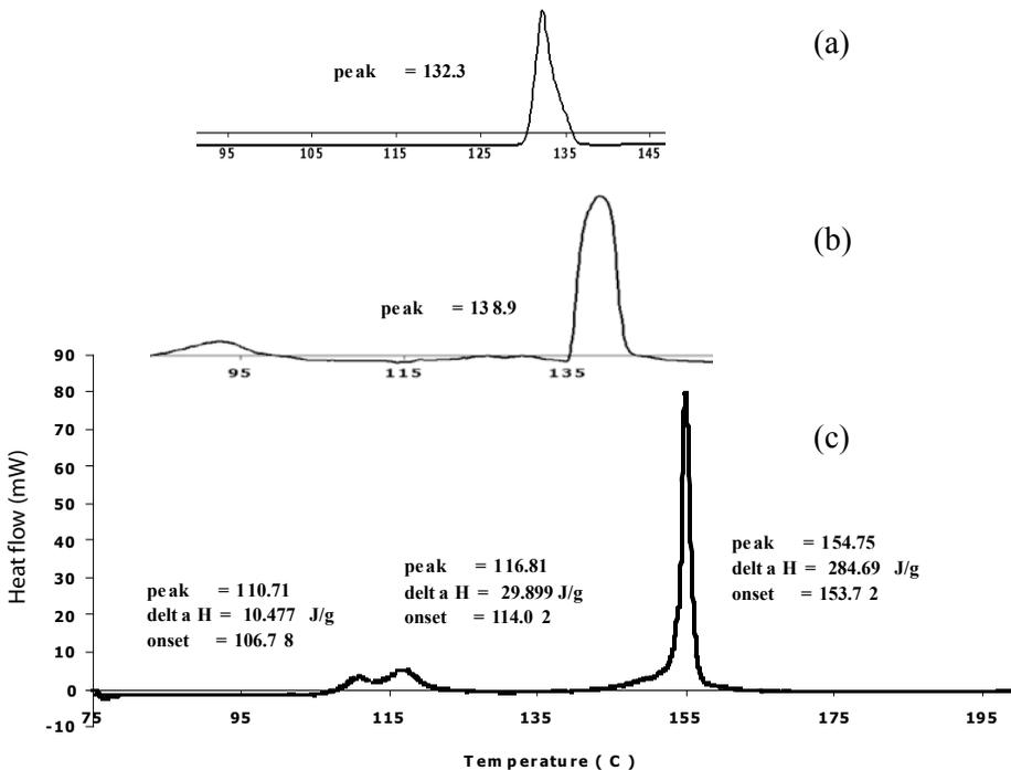
**Figure 8.** DSC thermograms of (a) diazepam, (b) DCP dihydrate and (c) powder scratched from the surface of DSDT prepared from DC blank tablet of 1000 kg CF. The curves have been separated in the y-axis to aid comparison.
