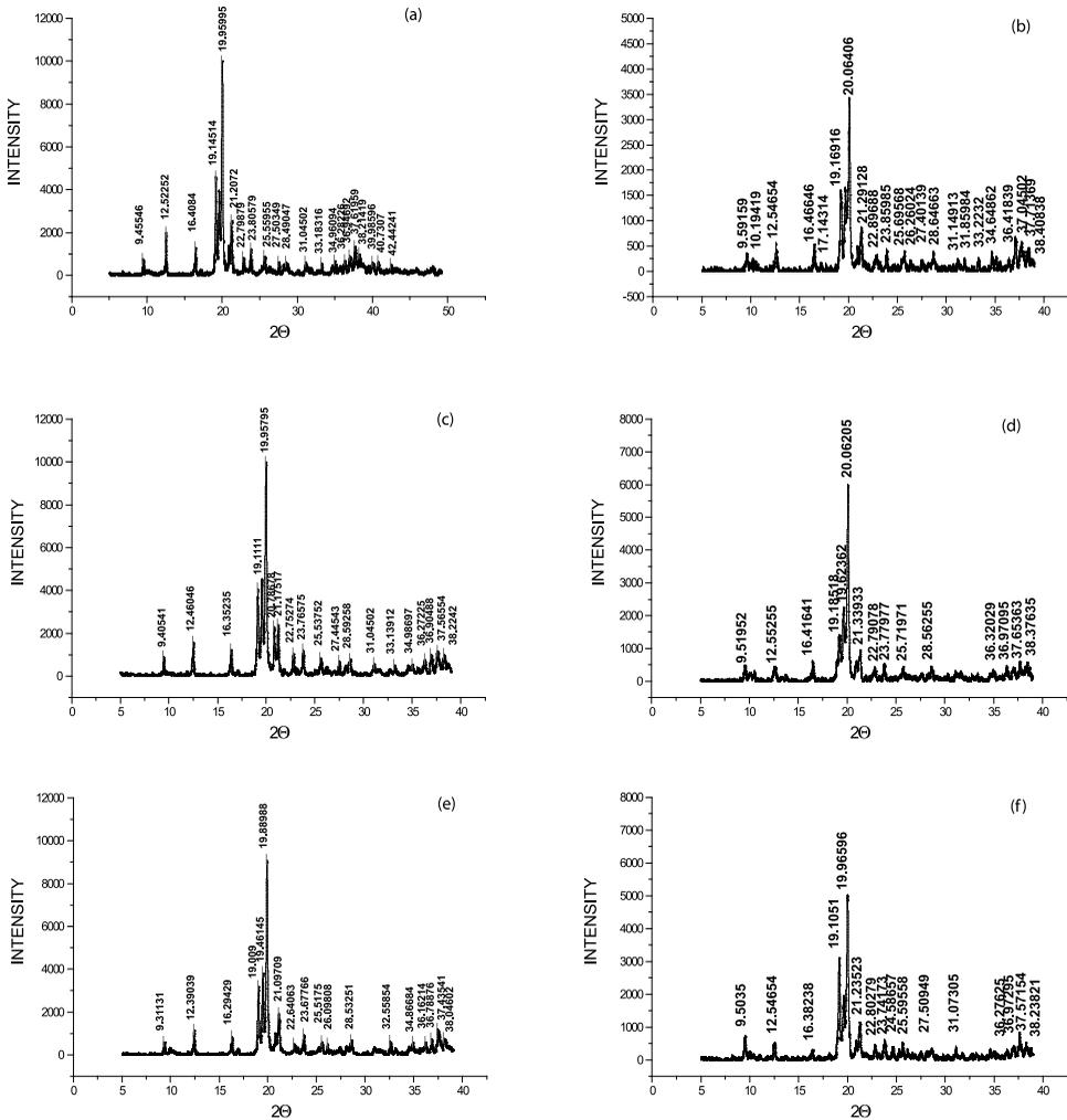
**Figure 7.** XRD patterns by X-ray monochromater of the powder scratched from the surface of WG blank tablet of 1000, 1400 and 1800 kg CF before dropping diazepam solution (a, c, e) and after dropping diazepam solution (d, b, f) of the same CF.
