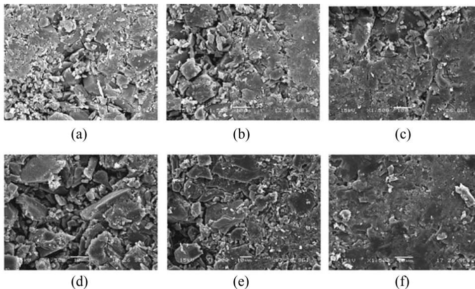
**Figure 2.** The surface morphologies by SEM (1,500X) of the DC blank tablets at CF of (a) 1000 kg, (b) 1400 kg and (c) 1800 kg and of DSDT prepared from DC blank tablet at (d) 1000 kg, (e) 1400 kg and (f) 1800 kg of CF.
