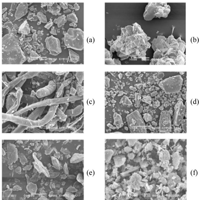
**Figure 1.** SEM morphologies (500X) of (a) Diazepam, (b) DCP dihydrate, (c) Ac-Di-Sol<sup>®</sup>, (d) Lactose (e) Talcum and (f) 1000X of Magnesium stearate.
