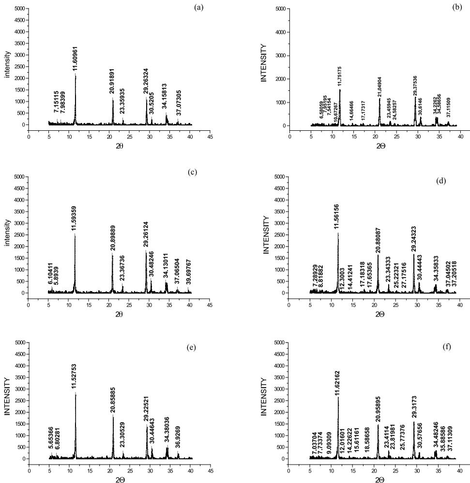
**Figure 6.** XRD patterns by X-ray monochromator of the powder scratched from the surface of DC blank tablet of 1000, 1400 and 1800 kg CF before dropping diazepam solution (a, c, e) and after dropping diazepam solution (b, d, f) of the same CF.
