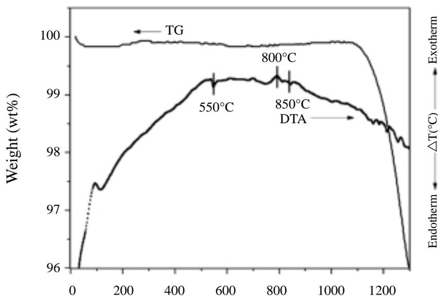
**Figure 1.** TG-DTA curves for the mixture of ZnO-Nb<sub>2</sub>O<sub>5</sub> powder.
