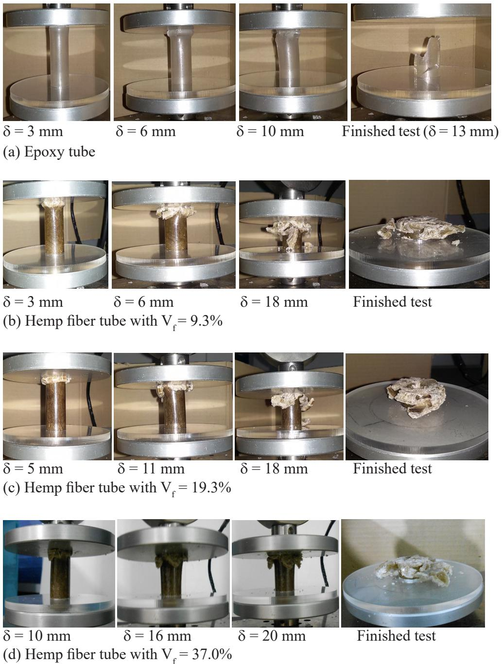
**Figure 2.** Failure mechanism of epoxy and hemp fiber tubes at different compressive displacements.
