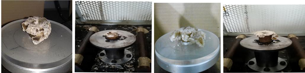
(c) Hemp fiber tube with  $V_f = 19.3\%$ (d) Hemp fiber tube with  $V_f = 37.0\%$
