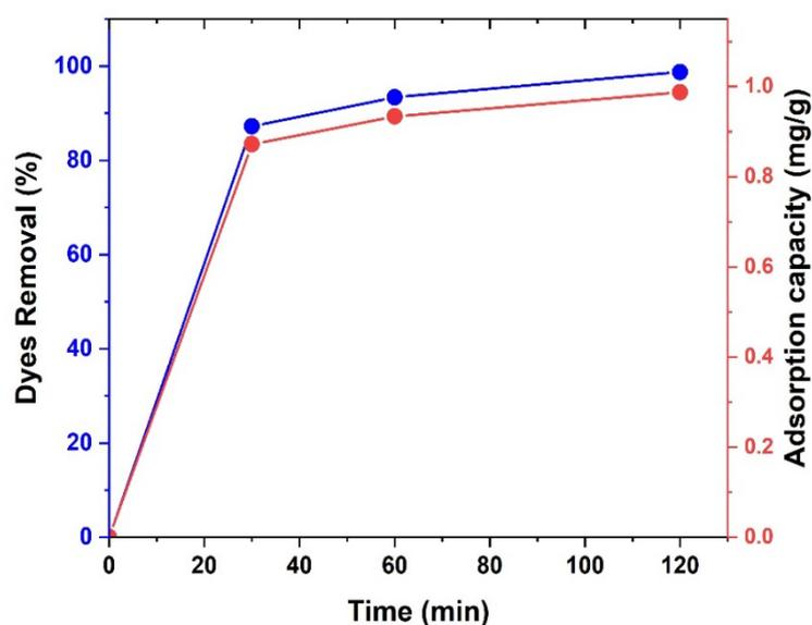
**Figure 11.** Removal efficiency of methylene blue in the water and adsorption capacity (mg/g)
