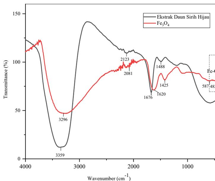
**Figure 4.** FTIR spectrum of  $\text{Fe}_3\text{O}_4$  (synthesized: green betel leaf extract).
