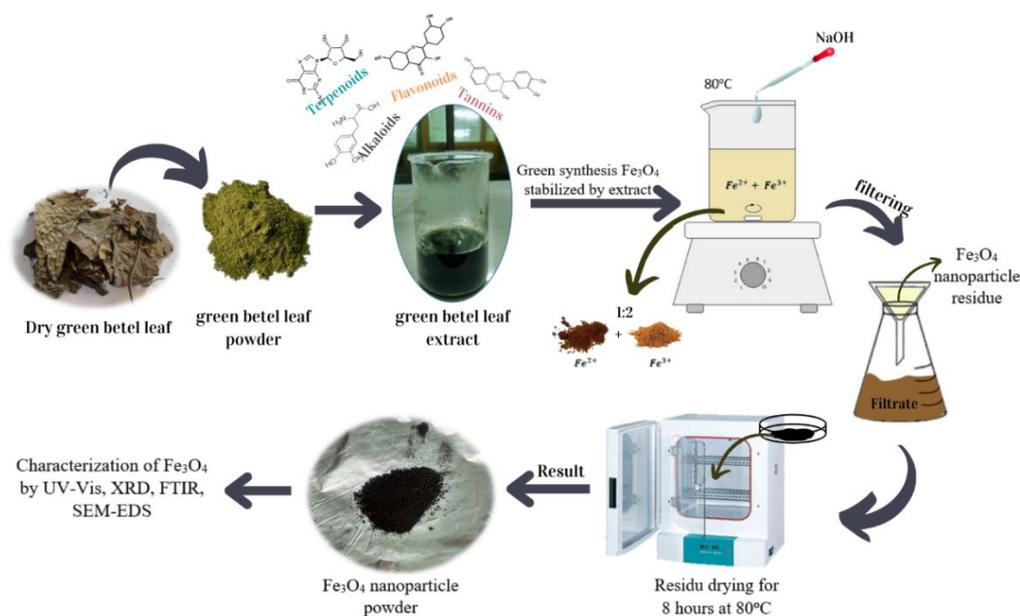
**Figure 1. Schematic of the synthesis of  $\text{Fe}_3\text{O}_4$  nanoparticles using the green synthesis method.**
