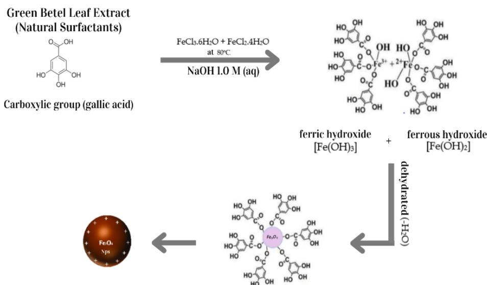
**Figure 10.** The mechanism of formation of  $\text{Fe}_3\text{O}_4$  nanoparticles uses a green betel leaf extraction solution.
