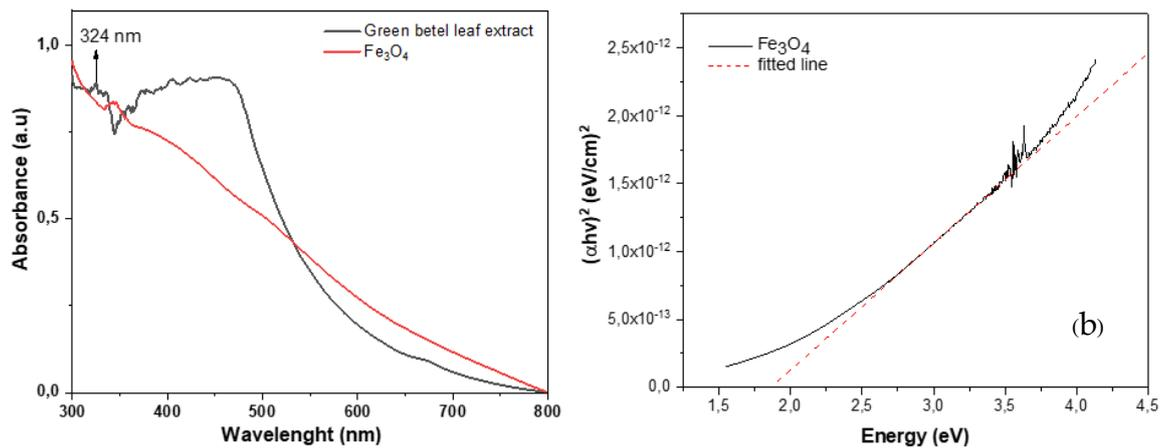
**Figure 2. (a) UV-Vis absorption spectra of green betel extract and Fe<sub>3</sub>O<sub>4</sub> nanoparticles (b) Band gap Fe<sub>3</sub>O<sub>4</sub> nanoparticles.**
