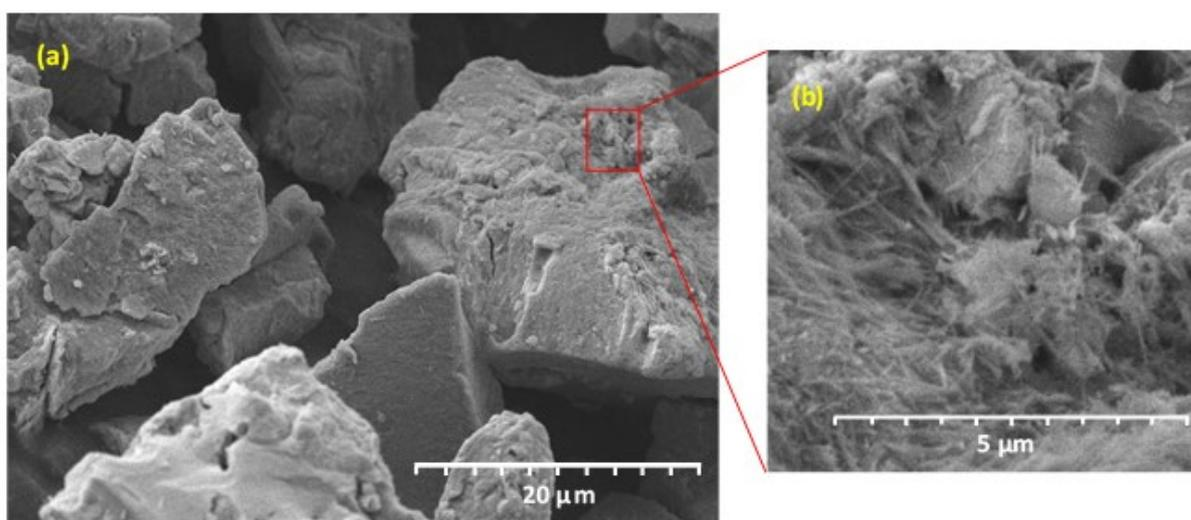
**Figure 5.** (a) Morphology of  $\text{Fe}_3\text{O}_4$  nanoparticles (b) Morphological magnification at  $5\text{ }\mu\text{m}$  (synthesized: green betel leaf extract).
