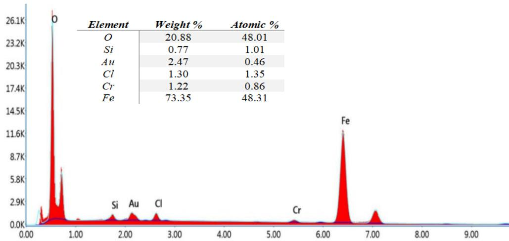
**Figure 7. EDS results from Fe<sub>3</sub>O<sub>4</sub> nanoparticles** (synthesized: green betel leaf extract).
