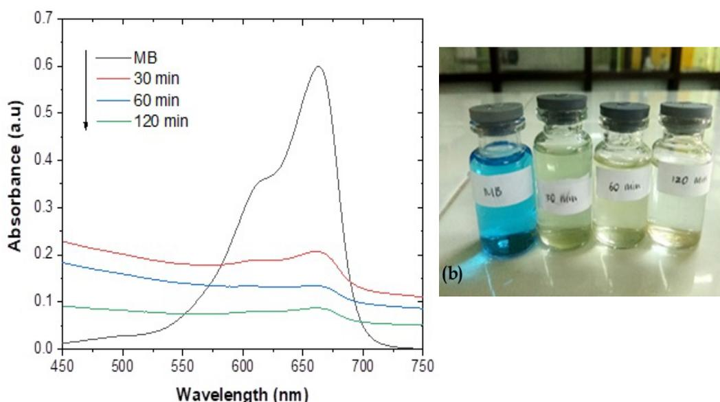
**Figure 9. (a) Absorption spectrum of UV-Vis adsorbed by time variation of  $\text{Fe}_3\text{O}_4$  nanoparticles (b) result of time variation of adsorption filtrate.**
