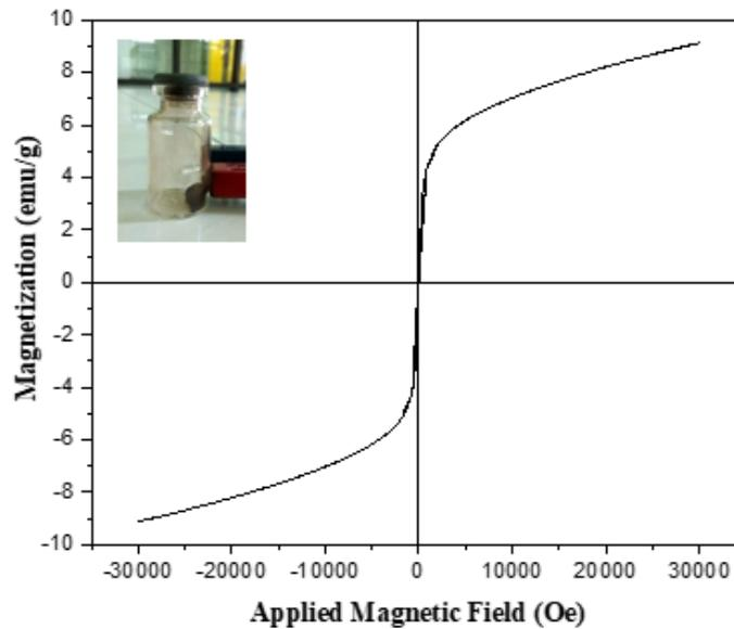
**Figure 8. Room temperature magnetization curve of Fe<sub>3</sub>O<sub>4</sub> nanoparticles** from green betel (*Piper betle* L.) leaf extract.
