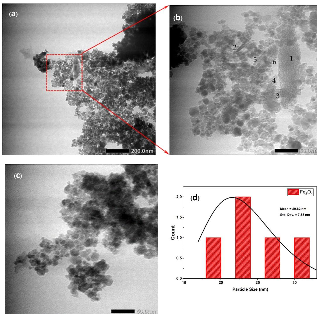
**Figure 6. HR-TEM morphology: (a-b) spherical and needle-like particles, (c) spherical particles, and (d) histogram of estimated size of  $\text{Fe}_3\text{O}_4$  nanoparticles that have been synthesized using green betel leaf extract.**
