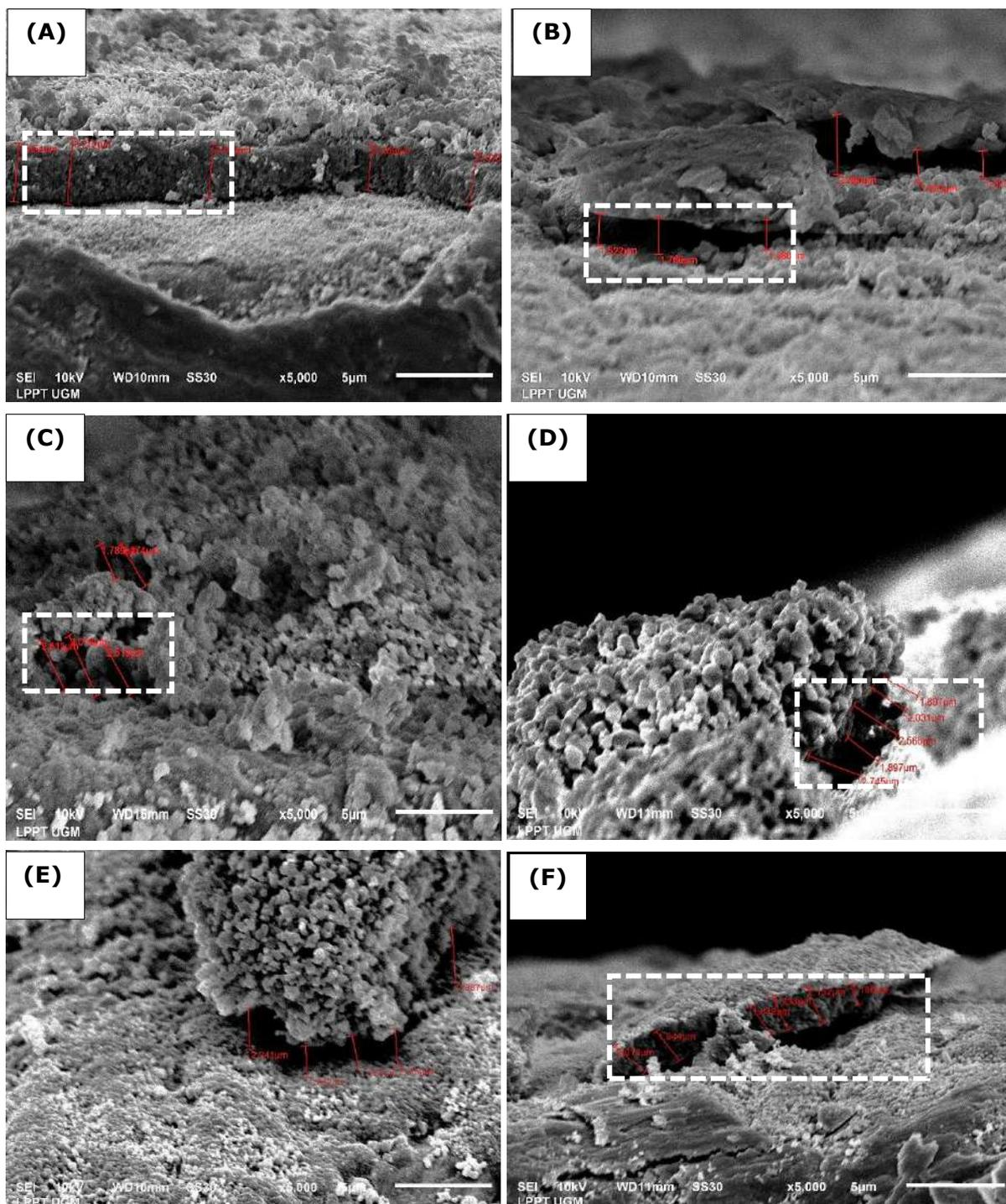
**Figure 2.** Cross-section of HA/Ti coating with variations of the withdrawal velocities, DC voltages, and calcination temperature of 750°C (A) 0.1 mm/s; 25V, (B) 0.1 mm/s; 50V, (C) 0.5 mm/s; 25V, (D) 0.5 mm/s; 50V, (E) 1 mm/s; 25V, and (F) 1 mm/s; 50V.
