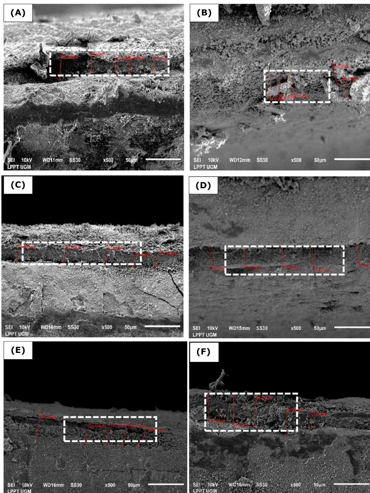
**Figure 3.** Cross-section of HA/Ti coating with variations of the withdrawal velocities, DC voltages, and calcination temperature of 950°C (A) 0.1 mm/s; 25V, (B) 0.1 mm/s; 50V, (C) 0.5 mm/s; 25V, (D) 0.5 mm/s; 50V, (E) 1 mm/s; 25V, and (F) 1 mm/s; 50V.
