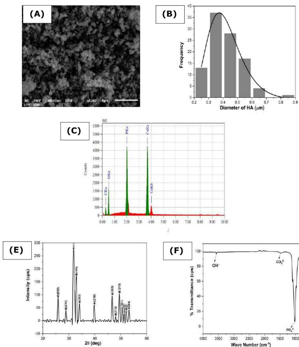
**Figure 1.** Physicochemical analysis of hydroxyapatite (A) morphology, (B) particle size distribution, (C)EDS analysis, (D)FTIR spectra, and (E)XRD pattern.
