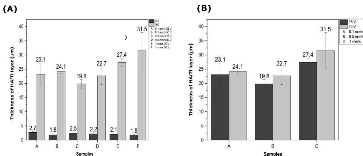
**Figure 4. (A) Effect of calcination temperatures on the thickness of HA/Ti layer and (B) effect of DC voltages on the thickness of HA/Ti layer.**
