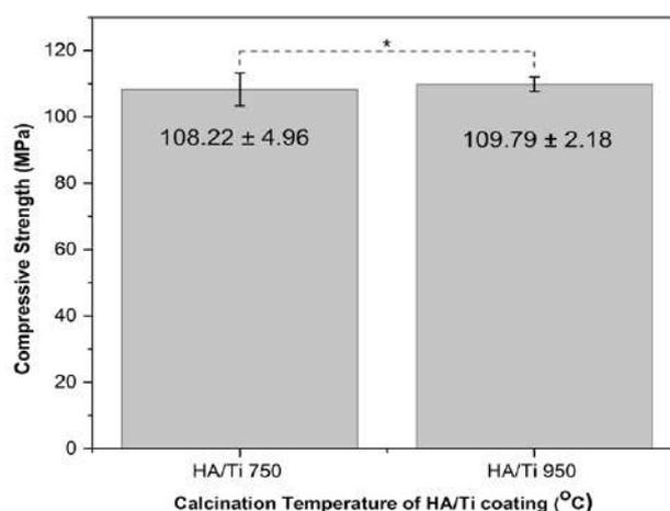
**Figure 7.** The average compressive strength value of HA/Ti coating with calcination temperatures of 750°C and 950°C (\*:  $P > 0.05$ ).
