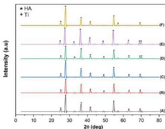
**Figure 6.** XRD pattern of HA/Ti coating with calcination temperature of 950°C (A) 0.1 mm/s; 25 V, (B) 0.5 mm/s; 25 V, (C) 1 mm/s; 25 V, (D) 0.1 mm/s; 50 V, (E) 0.5 mm/s; 50 V, and (F) 1 mm/s; 50 V.
