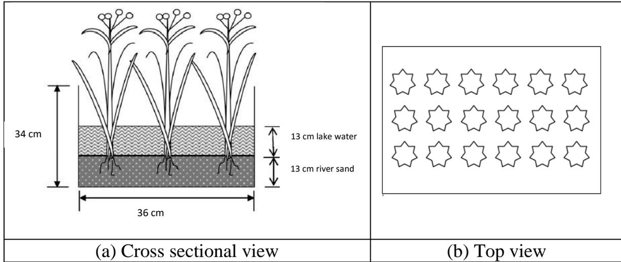
**Figure 1.** CW set up.
