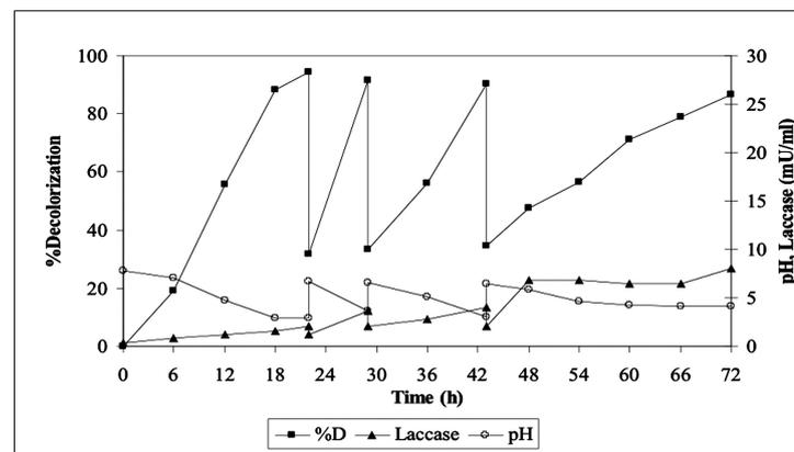
**Figure 1.** Profile of synthetic dye decolorization using immobilized *C. versicolor* RC3 on PUF in 10-liter air-bubble bioreactor.
