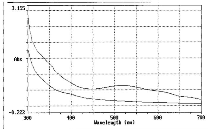
**Figure 3.** Wavelength scanning of real wastewater from Batik factory before (A) and after decolorization (B).
