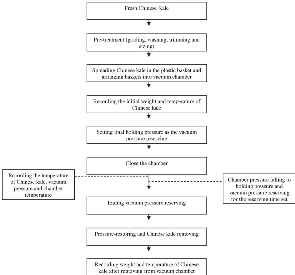
Figure 2. Flow chart of the vacuum cooling process.
