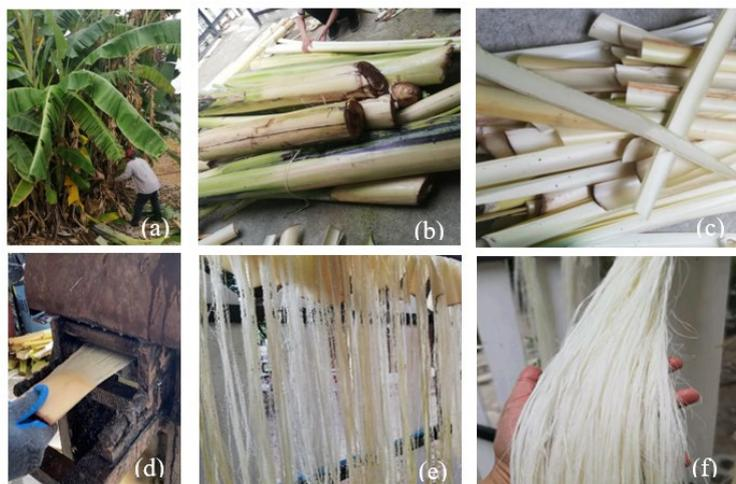
**Figure 1.** Illustrates the process of separating fibers from banana trunks: (a) Banana tree, (b) Banana tree trunk, (c) Leaf sheath of banana tree, (d) Fiber extraction using a semi-automatic separating machine, (e) Drying the fiber in the shade, (f) Obtained fiber.
