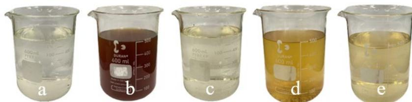
**Figure 2. Materials for treating banana fibers: (a) clean water, (b) ash-based solution, (c) drilling mud, (d) tamarind juice, (e) lemon juice.**
