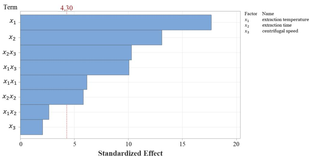
**Figure 1.** Pareto chart showing the order of significance of factors with yield as the response variable;  $\alpha = 0.05$
