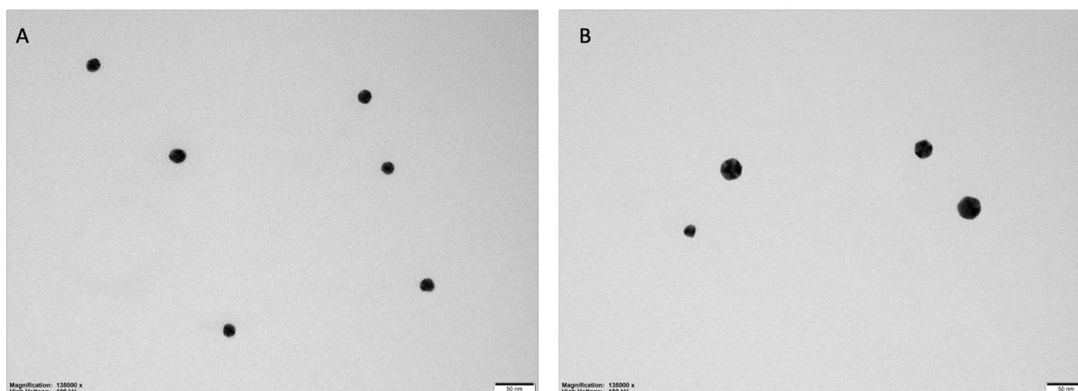
**Figure 1.** TEM images of (A) Ci-AuNPs and (B) CS-AuNPs at 135k × magnification.
