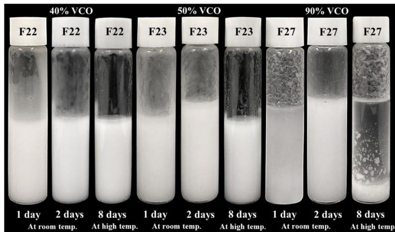
**Figure 2.** Stability evaluation of the selected CDC formulas with 0.3%w/v Aquagel™ 45 at one and two days of incubation at room temperature, and after eight days of extreme thermal incubation.
