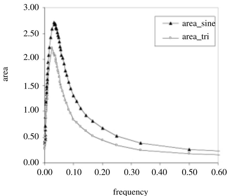
**Figure 2.** Simulated area of hysteresis loop A being driven by the sinusoidal magnetic field (—▲—: area\_sine) and the triangular magnetic field (—□—: area\_tri) as a function of frequency  $f$  plotted at a fixed amplitude ( $h_0 = 1 J$ ) and a fixed temperature ( $T = 2.6 J/k_B$ ).
