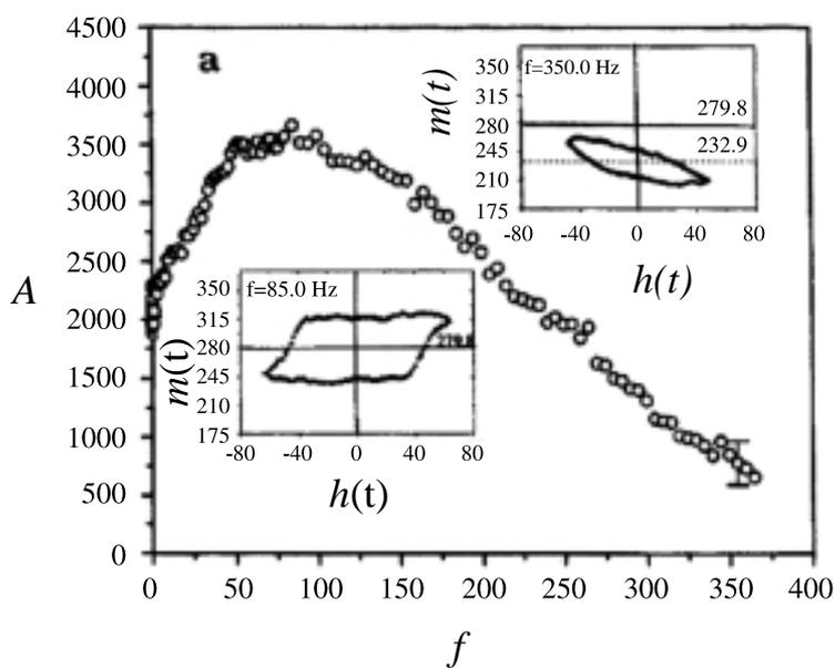
**Figure 3.** After Jiang et al., (1995), experimental results on the dynamic hysteresis loop-area as a function of frequency at a fixed ac current of 0.4 Amp. The direction of the magnetic field is parallel to the film plane. The insets show plots of  $m$ - $h$  loop for the following particular values of the field amplitudes  $h_0$  : (i)  $h_0 = 48.0$  Oe (top inset) and (ii)  $h_0 = 63.0$  Oe (bottom inset).
