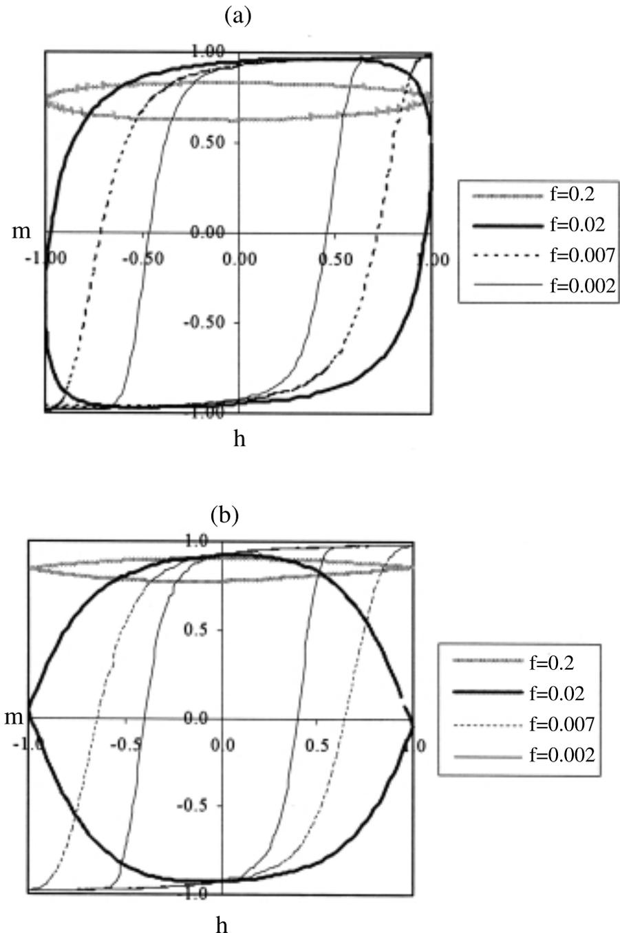
**Figure 1.** Simulated hysteresis loops being driven by (a) sinusoidal magnetic field and (b) triangular magnetic field at various frequencies  $f$  (in the  $\text{mcs}^{-1}$  unit) but fixed amplitude of the external magnetic field ( $h_0 = 1.0 J$ ) and a fixed temperature  $T = 2.0 J/k_B$ .
