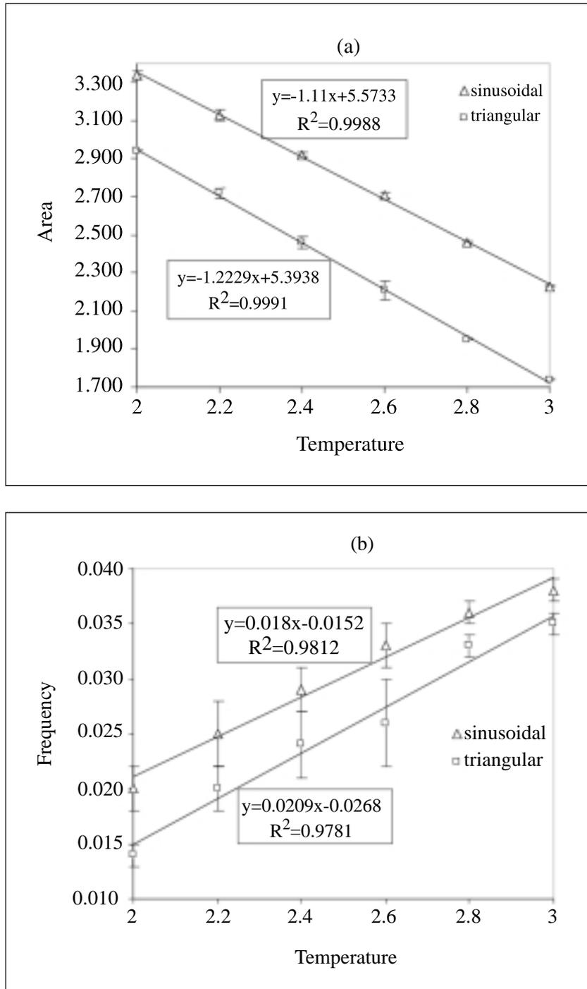
**Figure 4.** (a) Maximum area of hysteresis loop and (b) the frequency at the maximum area of the Ising system being driven by the sinusoidal magnetic field and the triangular magnetic field as a function of temperature plotted at a fixed amplitude  $h_0 = 8$  J. Solid lines are the linear fits to the results.
