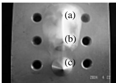
**Figure 3.** The accumulation of PAN fibers derived from the spinning at the position 2 cm from the center of metal plate and the spinning height of 10 cm.
