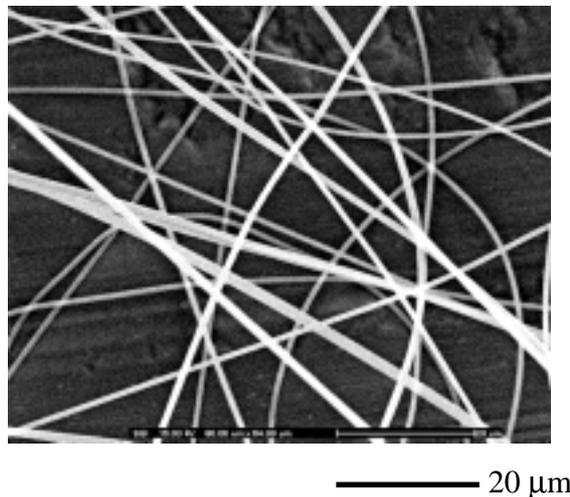
**Figure 5.** SEM micrograph of resultant PAN nanofibers. The fibers were spun at a flow rate of 0.1 ml/min and a voltage of 20 kV with a standard nozzle from a 12% (w/v) N,N-dimethylformamide solution.
