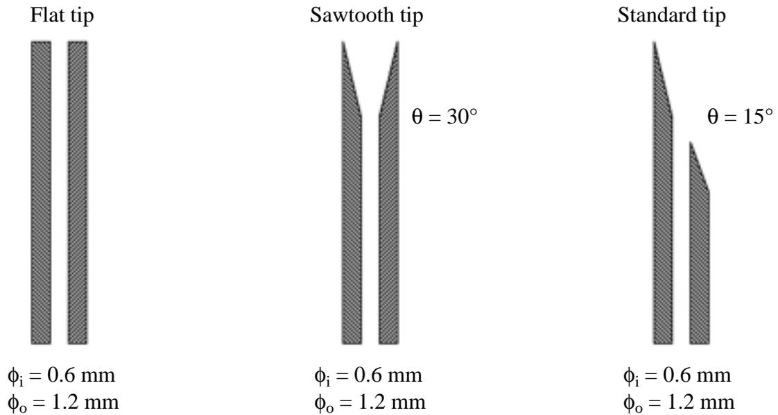
**Figure 2.** Geometry of three nozzles for the feeding of PAN solution. ( $\phi_i$  = inner diameter,  $\phi_o$  = outer diameter).
