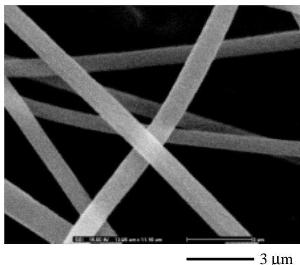
**Figure 5.** SEM micrograph of electrospun PAN fibers. The fibers were spun from a 12 wt% solution of PAN in *N,N*-dimethylformamide at a flow rate of 0.1 ml/min and a voltage of 20 kV with a flat nozzle.
