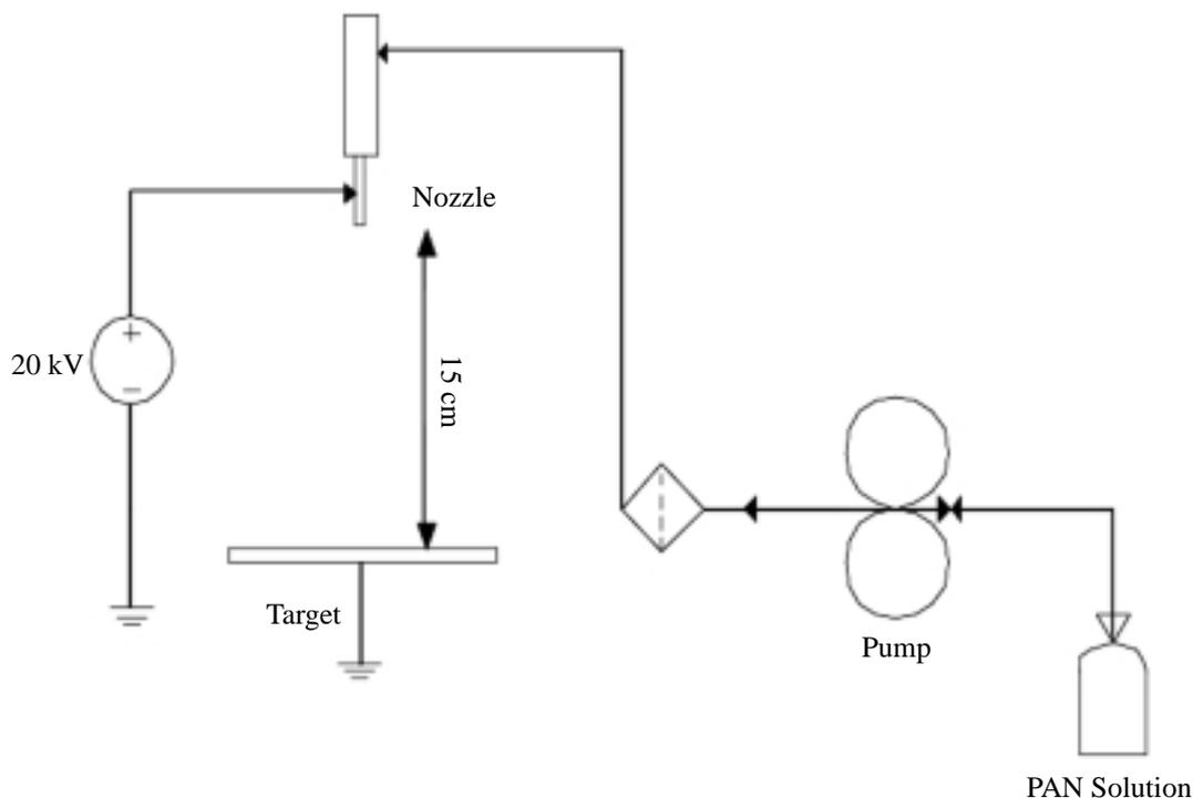
**Figure 1.** Schematic view of the electrospinning setup.
