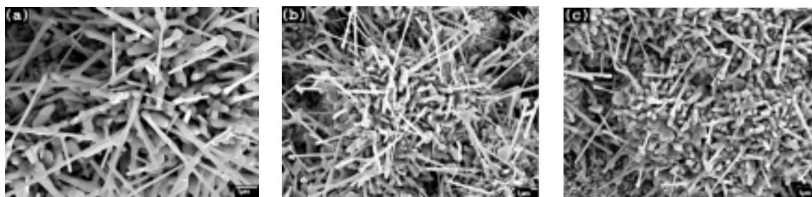
Figure 2. FE-SEM images of ZnO nanostructures grown at (a) 600°C, (b) 700°C and (c) 800°C for 24 hr.
