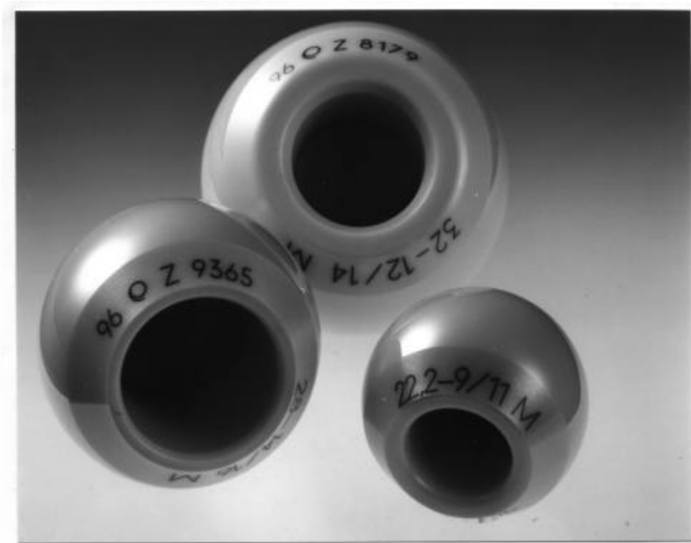
Figure 4. Laser markings of zirconia femoral ball heads (Heimann and Willmann, 1999).
