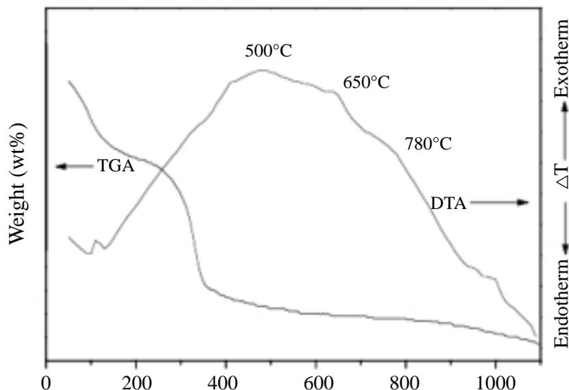
**Figure 1.** TG-DTA curves for the mixture of MgO-Nb<sub>2</sub>O<sub>5</sub> powder.
