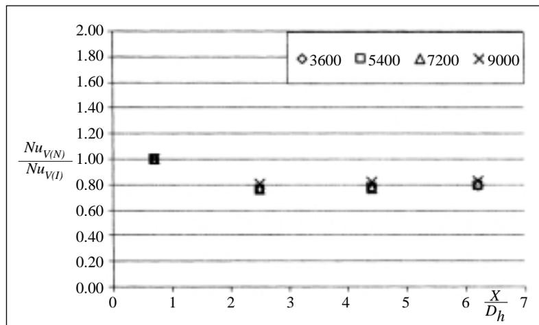
**Figure 6.** The ratio of adiabatic Nusselt number at different positions to that at the first row at various values of  $\frac{X}{D_h}$  and different attack angles. There was a set of vortex generators integrated in front of the first row only.
