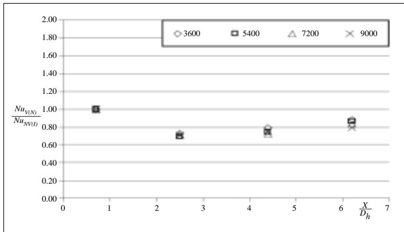
**Figure 5.** The heat transfer enhancement in terms of adiabatic Nusselt numbers with and without vortex generators. The vortex generators were integrated in front of the first row only. The attack angle was 20 degree.
