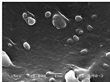
**Figure 4.** SEM image of dried nanoparticles of MPEG5,000-PDLL prepared by using 3/1 (v/v) acetone/ethanol mixture solvent (bar = 1,000 nm).
