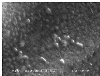
**Figure 3.** SEM image of dried nanoparticle aggregates of MPEG5,000-PDLL prepared using 3/1 (v/v) acetone/ethanol as the mixture solvent (bar = 500 nm).
