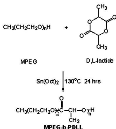
**Figure 1.** Polymerization reaction of MPEG-*b*-PDLL.
