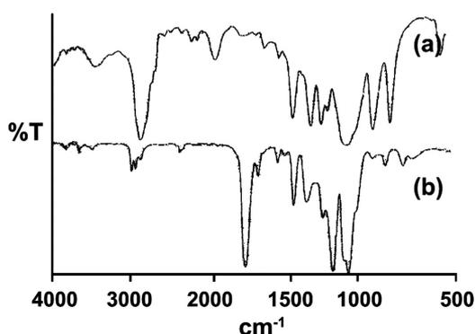
**Figure 2.** FTIR spectra of (a) MPEG5,000 and (b) MPEG5,000-PDLL.
