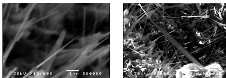
**Figure 2.** Show the width of nanobelts of products.
