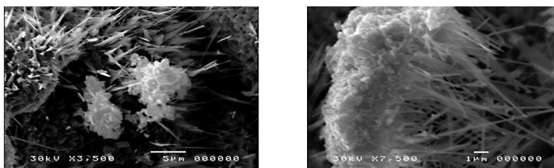
**Figure 1.** Scanning electron microscope images of Zn nanobelts.
