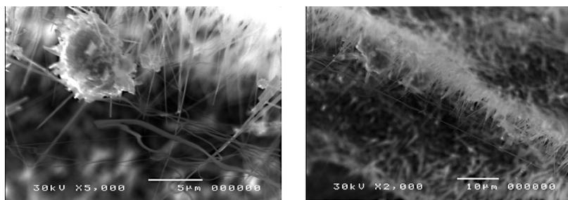
**Figure 3.** Scanning electron microscope images of Zn nanowires.
