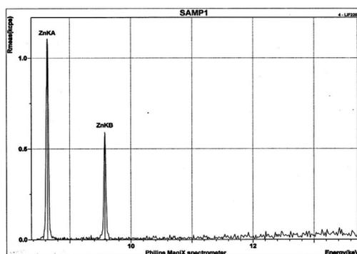
**Figure 4.** Wavelength dispersive X-ray fluorescent (WDXRF) pattern of metallic Zn nanowires. No other peak is shown except for the Zn.
