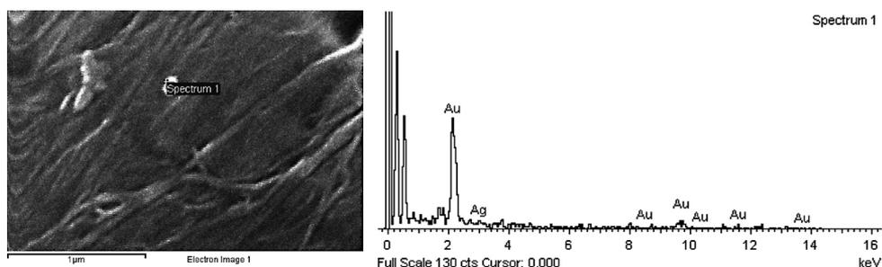
**Figure 2.** The EDS analysis of silver nanoparticles finished cotton fiber.
