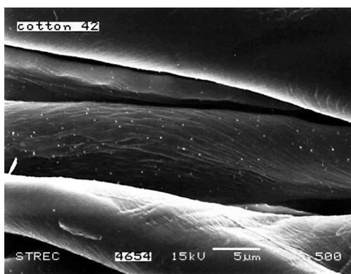
**Figure 1.** SEM micrograph of silver nanoparticles on cotton fabric.
