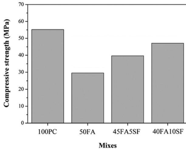
**Figure 4.** Compressive strength of Portland cement, binary and ternary blended cement mortars at 50% replacement.
