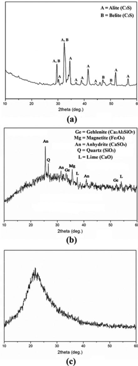
**Figure 1.** XRD patterns of materials used in this research (a) Portland cement (b) fly ash and (c) silica fume.
