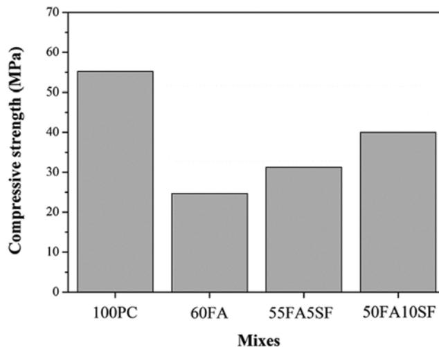
**Figure 5.** Compressive strength of Portland cement, binary and ternary blended cement mortars at 60% replacement.
