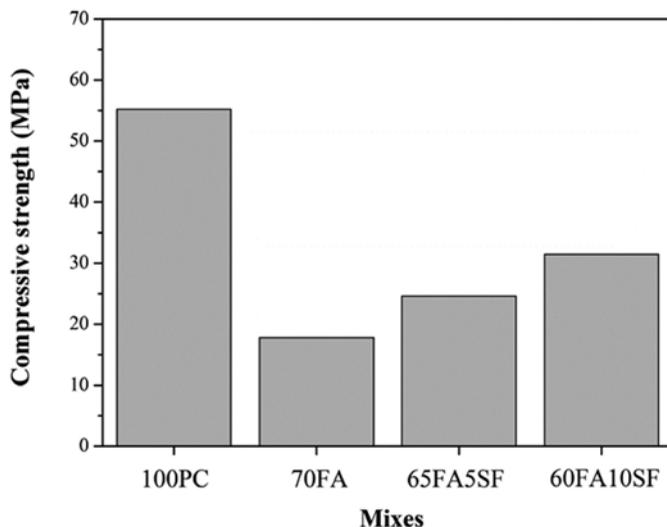
**Figure 6.** Compressive strength of Portland cement, binary and ternary blended cement mortars at 70% replacement.
