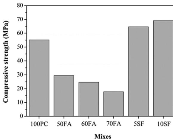
**Figure 3.** Compressive strength of Portland cement and binary blended cement mortars.
