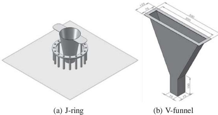
**Figure 3.** Slump flow, J-ring test and V-funnel test apparatus.
