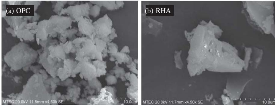
**Figure 1.** Scanning electron micrographs (4500x) of (a) Ordinary Portland Cement and (b) rice husk ash.
