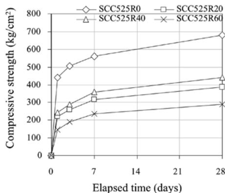
**Figure 4.** Compressive strength of self-compacting concrete.
