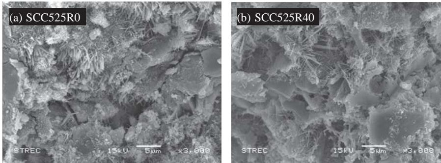
**Figure 5.** Scanning electron micrographs (3000x): (a) SCC525R0 and (b) SCC525R40.
