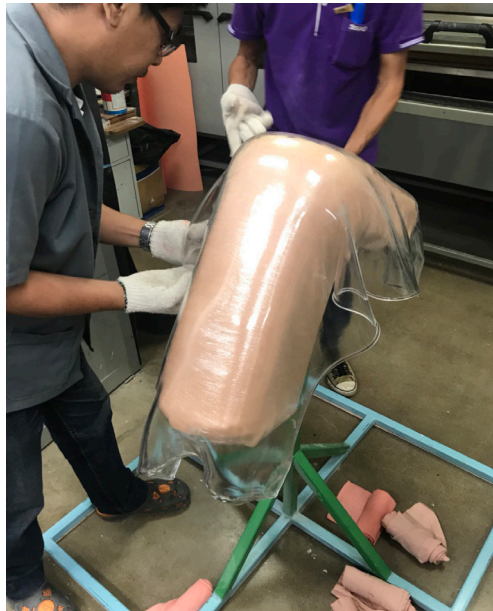
Figure 1. Image taken during fabrication of patients custom seating orthosis.
